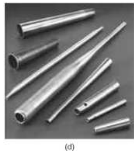
FIGURE 14.14 (a) Schematic illustration of the rotary-swaging process. (b) Forming internal profiles on a tubular workpiece by swaging. (c) A die-closing swaging machine, showing forming of a stepped shaft. (d) Typical parts made by swaging. Source: (d) Courtesy of J. Richard Industries.
