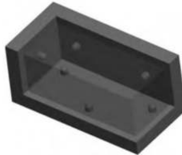
Fig. 6.2 Six point location of a rectangular block
