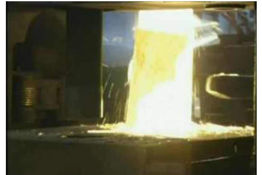
(a) Ideal deformation of a solid cylindrical specimen compressed between flat frictionless dies (platens), an operation known as upsetting.
